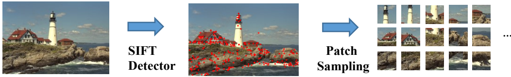
Figure 4.1: Patch extraction using interest point sampling strategy
