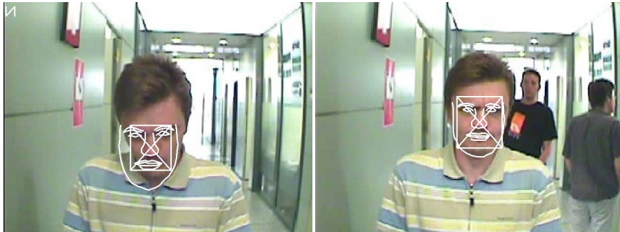
Figure 4.2: Examples of bad (left) and good (right) facial segmentation. Including inaccurately segmented images corrupts the training set.
