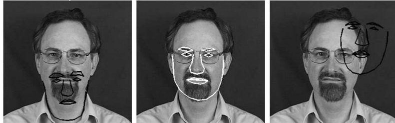
Figure 5.1: Three examples of ASM matches to a face image. Two of them (in dark color) are clearly wrong (e.g. due to a bad initialization).
