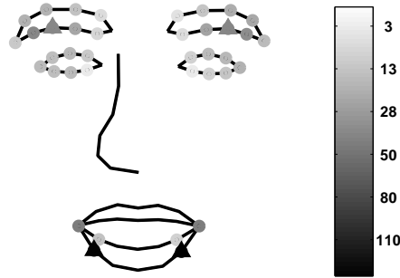
Figure 4.4: Best four points for the estimation of homographies in left-right head rotation (triangles). Other points included within the 200 best subsets of four points are also shown (circles). The different colors indicate the number of times that each point was selected within the best 200 subsets, according to the scale indicated on the right.
